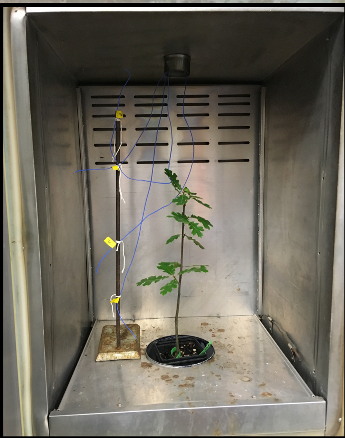
A Black Oak ( Q. kelloggii ) seedling placed within a customized laboratory oven used to simulate a 100°C heat plume.
