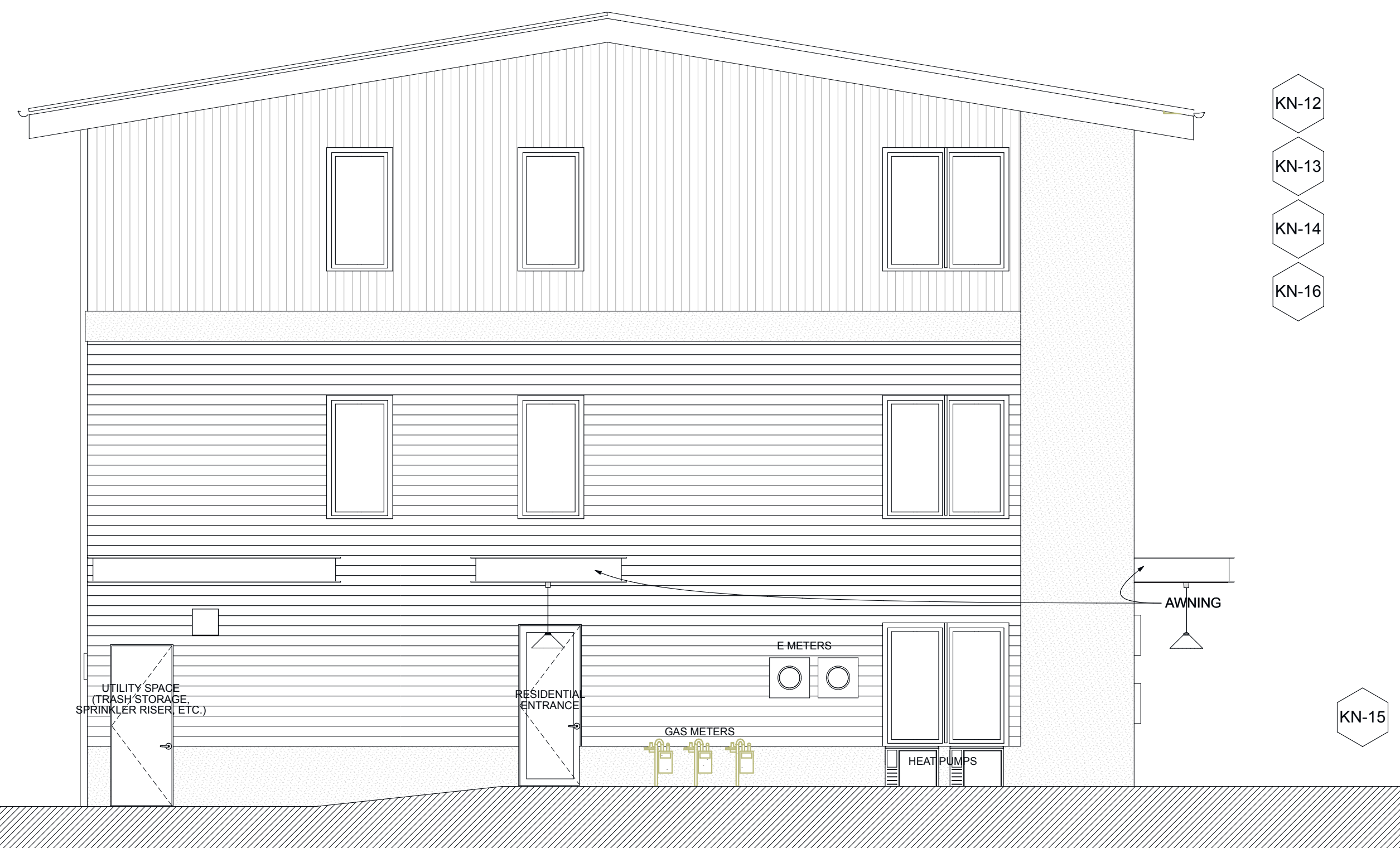
2 LEFT ELEVATION SCALE: 3/16" = 1'-0"
