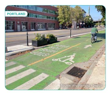
In areas separated from motor vehicle lanes, e-scooter stencils are used to indicate to e-scooter riders where to travel. Scooter symbols on signs or markings are considered experimental under the 2009 U.S. Manual on Uniform Traffic Control Devices (MUTCD), so jurisdiction-by-jurisdiction decisions are made about whether to include them in mixed traffic conditions or to limit their application to separated bikeways.
