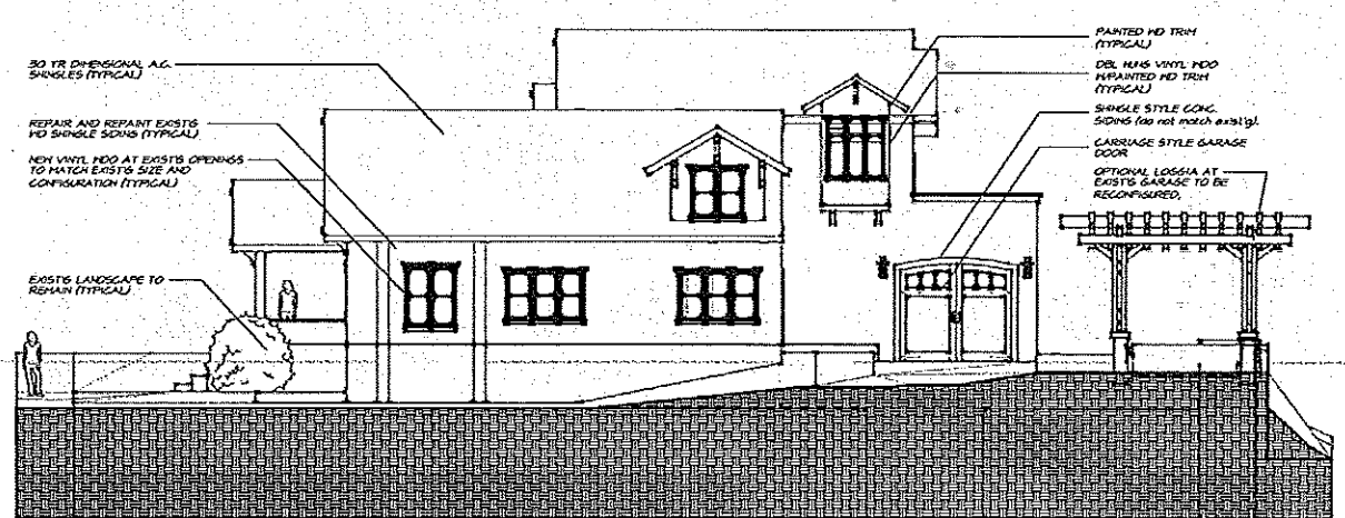
143 EAST ELEVATION SCALE: 1/8"=1'-0"
