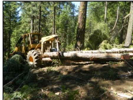
Used to skid logs to the log landing and to drag slash onto skid trails for restoration.
