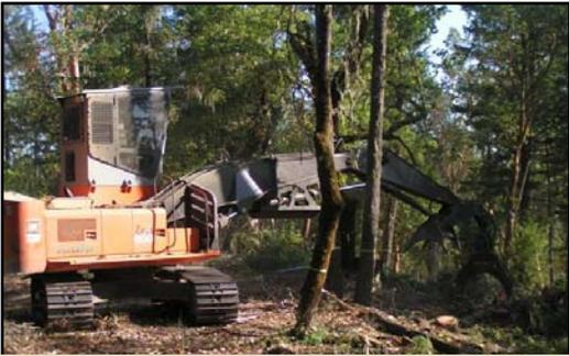
Used for pulling logs from the forest onto the road and loading logs onto log trucks.
