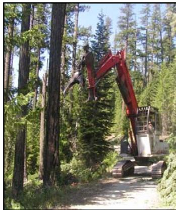
Used to pull logs onto established skid trails.
