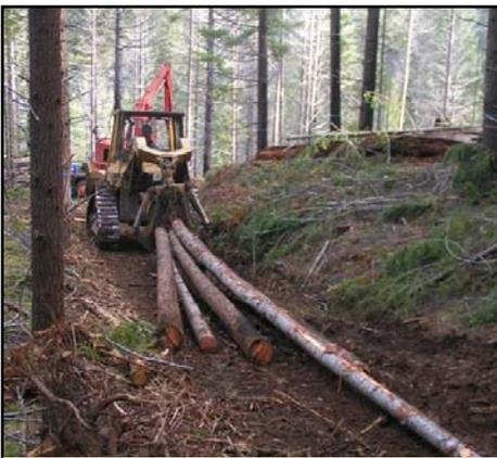
Used to move logs to log landings and clear debris.
