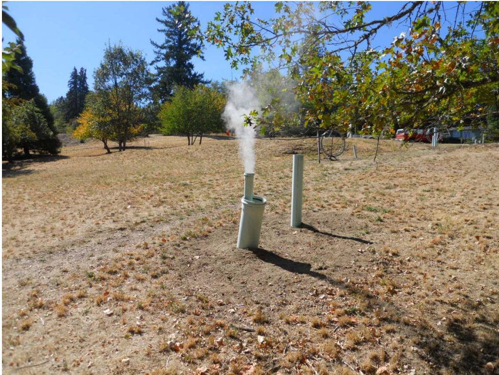
Southern most end of SOU: Smoke emitting from missing cleanout cap
