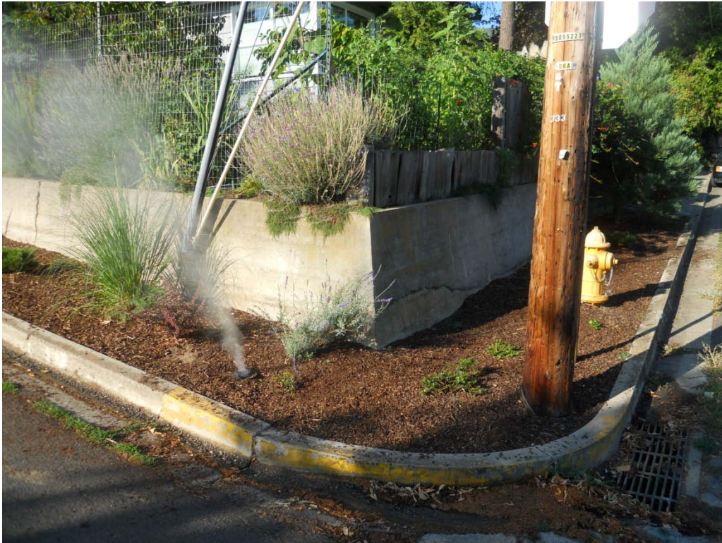
SW corner of Holly and Harrison: Smoke pouring out of broken cleanout cap
