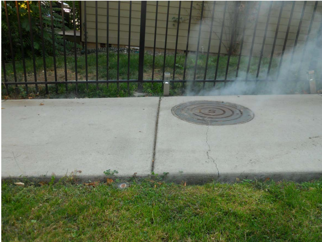
MH 09DD-005: Smoke seeping from crack in sidewalk and along edges of sidewalk near manhole
