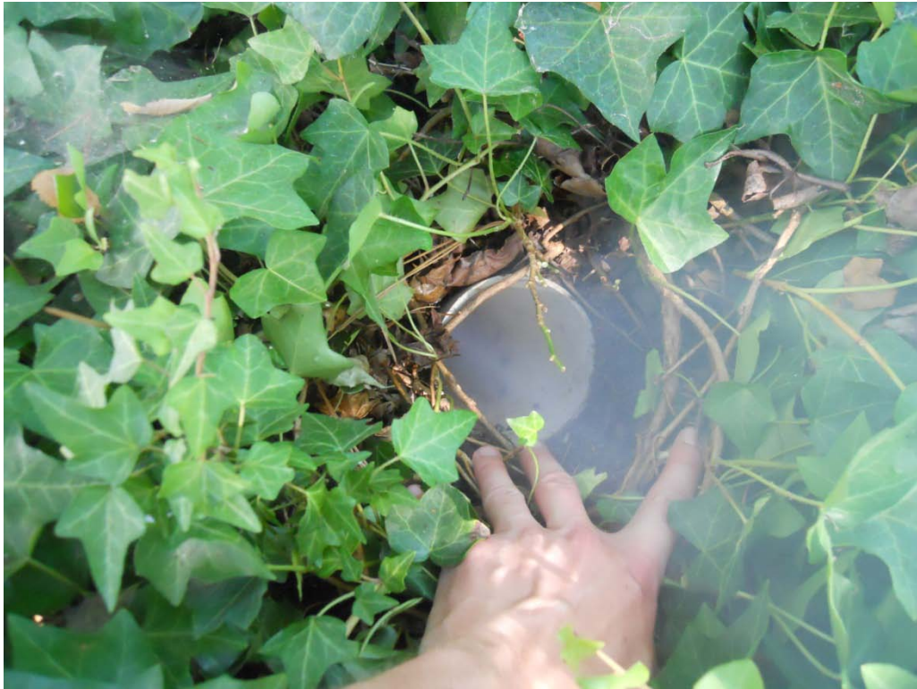
715 Pracht Street: Smoke emitting from cleanout missing cap
