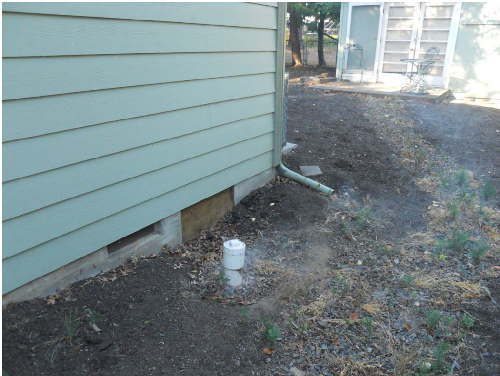
501 Beach Street: Smoke seeping from ground around cleanout near downspout splash block
