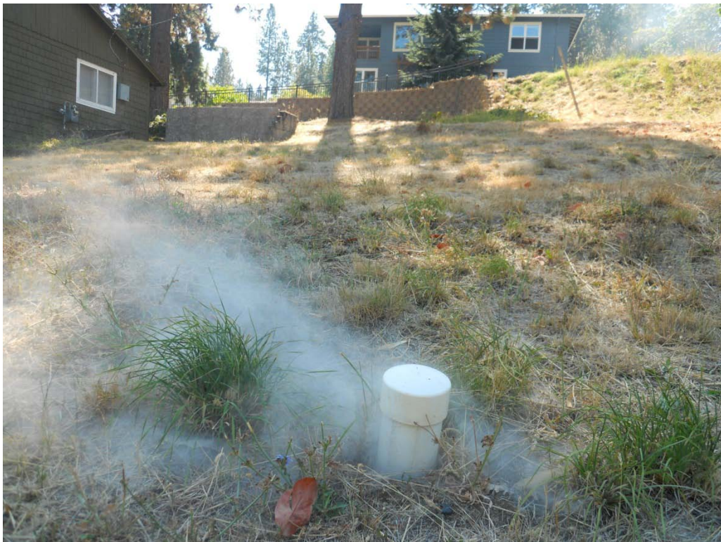
Vacant lot west of 759 Prospect Street: Service lateral stub smoking from ground
