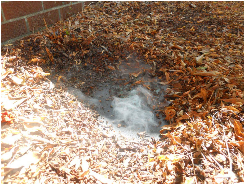
328 Liberty Street: Smoke emitting from unscrewed cleanout cap
