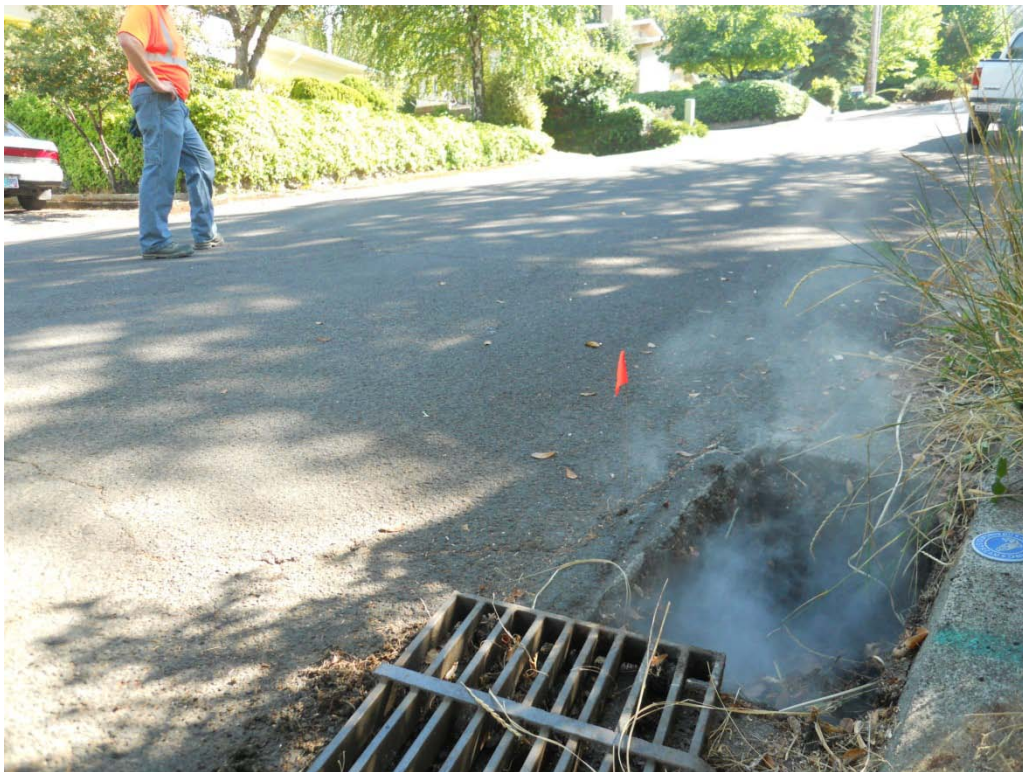
Catch basin in front of 645 Glenwood Drive: Smoke emitting from catch basin
