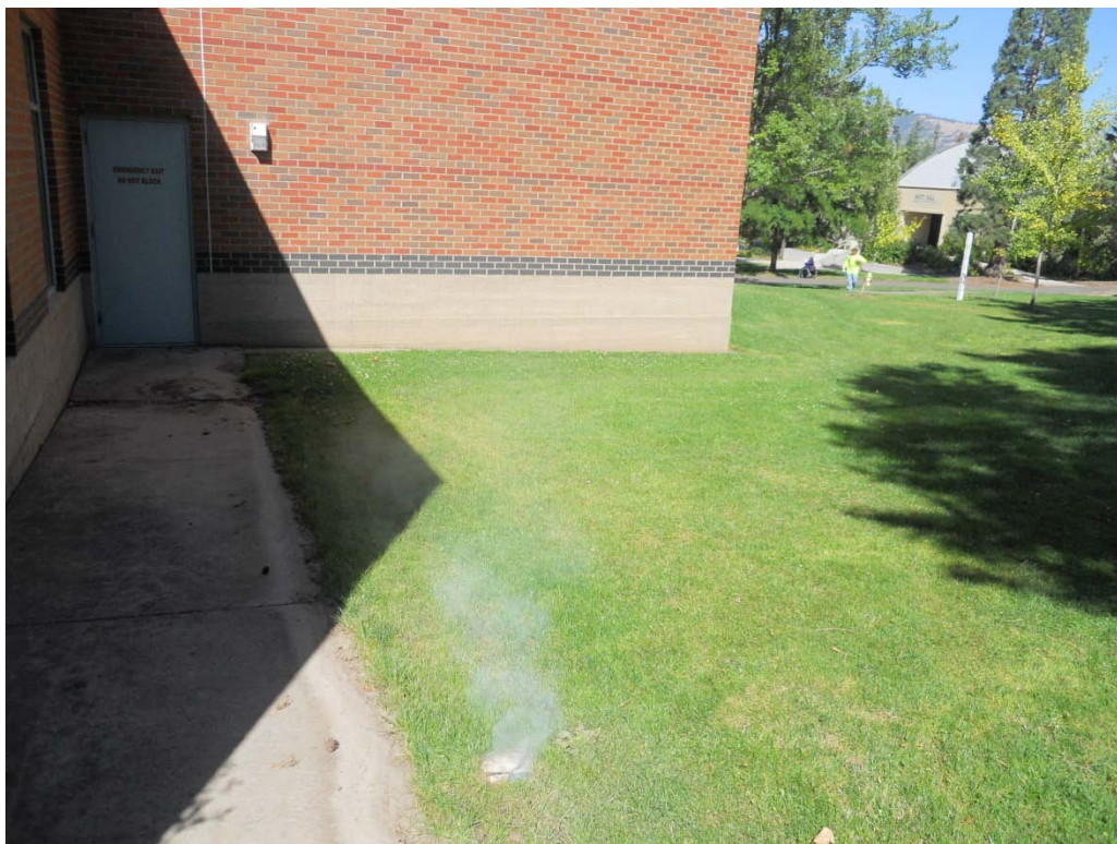
NW corner of Central Hall of SOU Campus: Smoke emitting from broken cleanout cap
