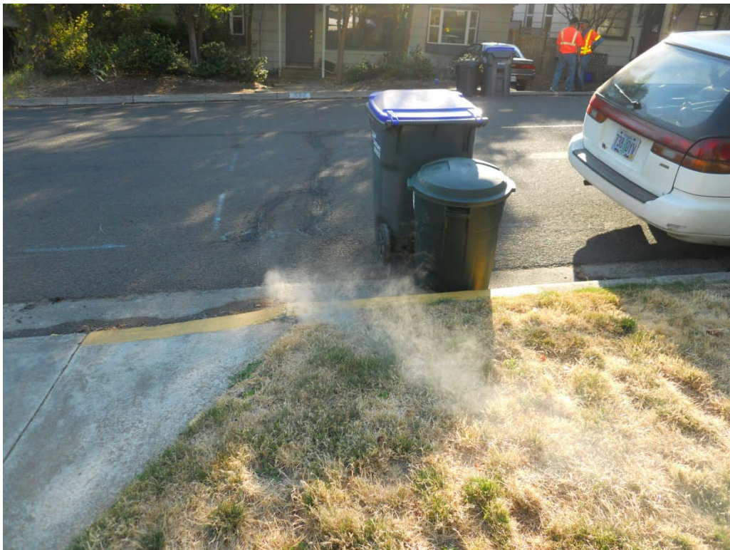
429 Beach Street: Smoke emitting from crack in curb and gutter
