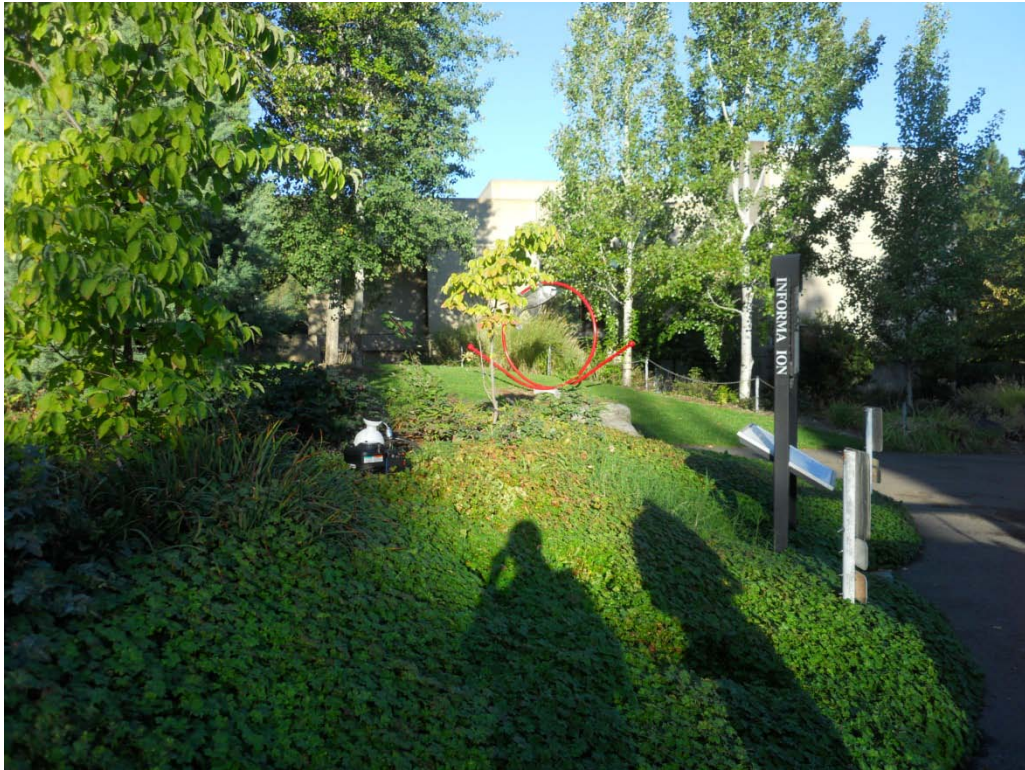
SOU Campus between MH 10CC-024 and 10CC-023: No smoke traveling between manholes, pipeline could be clogged
