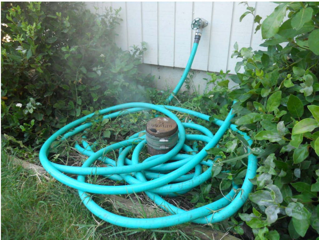
140 7 th Street: Smoke emitting from broken cleanout cap
