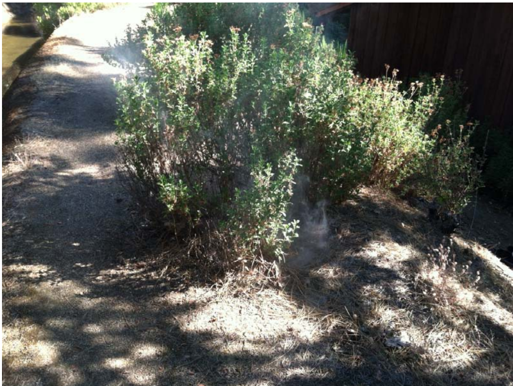
748 Lisa Ln: Smoke emitting from broken service lateral
