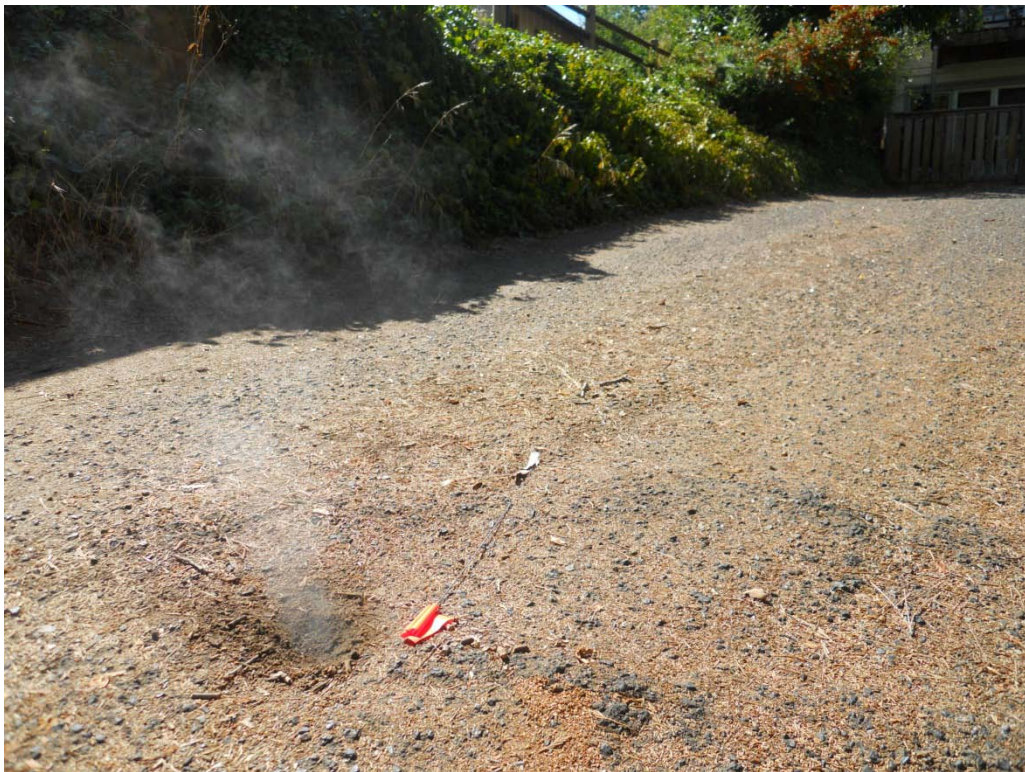
449 Morton Street: Smoke emitting from crack in driveway from tree roots
