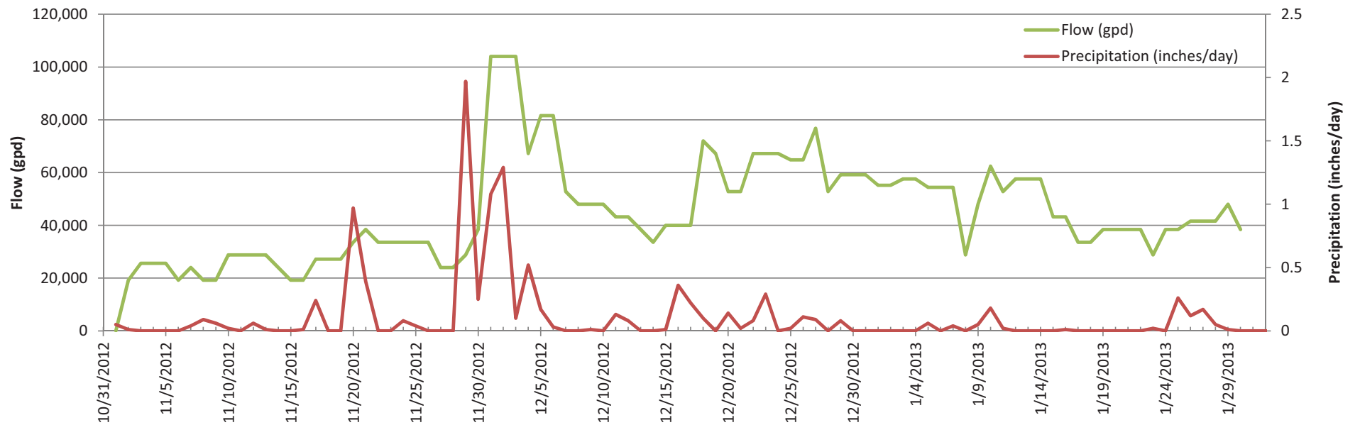
Grandview P.S.: Flow & Precipitation vs. Time
