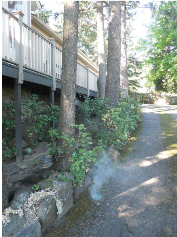
801 Clarence Way Driveway: Smoke emitting from cleanout missing cleanout cap
