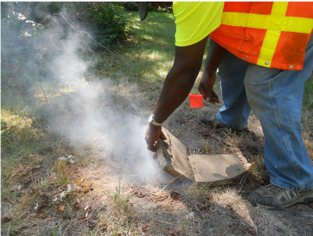
671 Mountain Avenue: Stones used in place of cleanout cap
