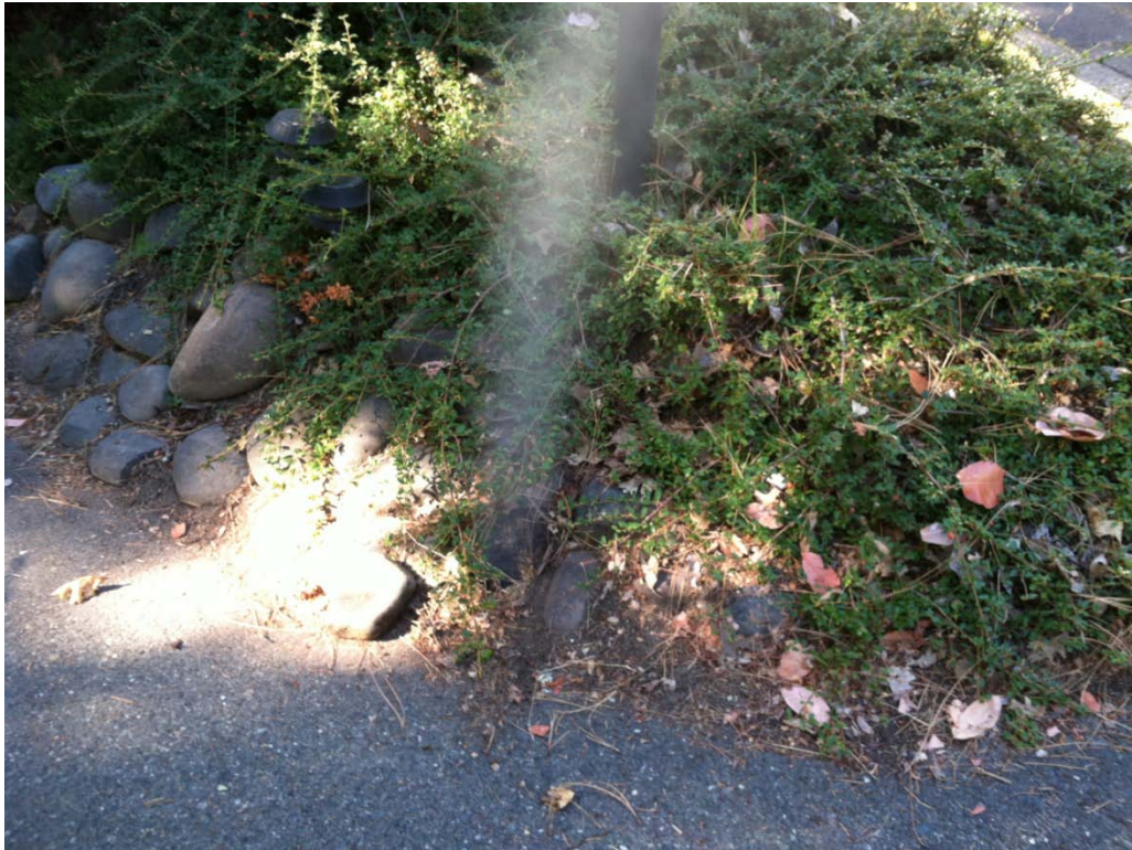
898 Morton St: Smoke emitting from missing cleanout cap
