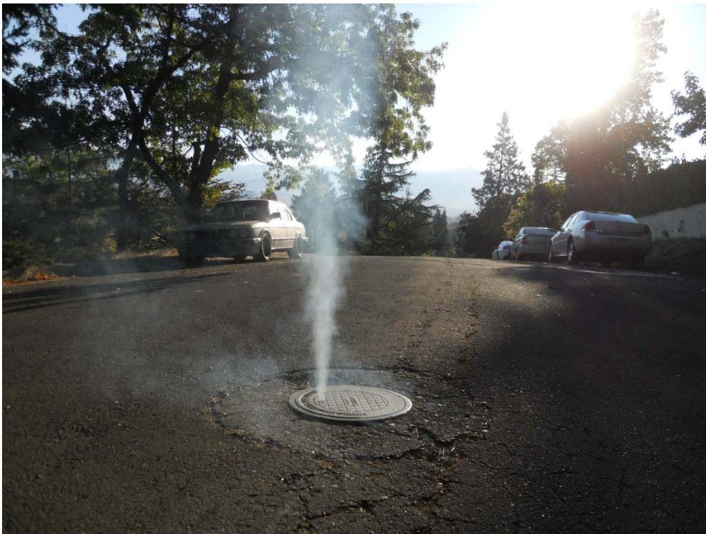
SE of Euclid Avenue and Pracht Street intersection: Smoke emitting from around the cleanout collar
