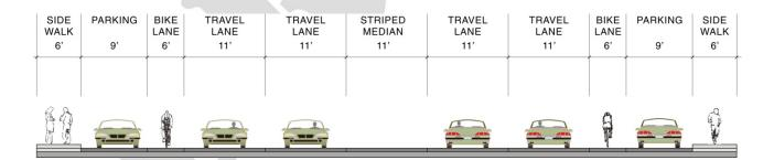
The following series of photos illustrate the previous 12<sup>th</sup> Street cross-section, the proposed road diet cross-section and the temporary cross-section implemented to test the concept. Exhibit 1 illustrates the "before" 7-lane cross-section on 12<sup>th</sup> Street approaching an intersection.
