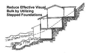
The top of cut slopes not utilizing structural retaining walls shall be located a minimum setback of one-half the height of the cut slope from the nearest property line.
