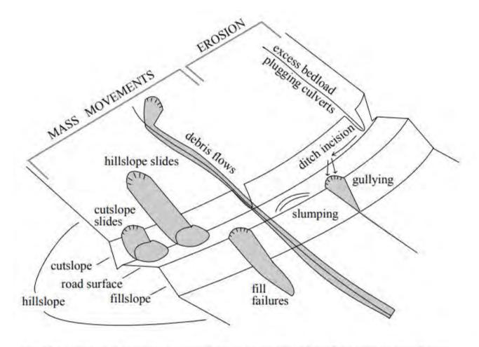
Figure 8.2. Eight types of road failures inventoried in the Lookout Creek and Blue River watershed (from Wemple et al., 2001).
