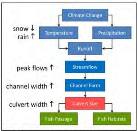
**Figure 2.** Causal relationships between culverts and climate change. Climate change is projected to increase the proportion of precipitation that falls as rain rather than as snow. As a result, winter peak flows in western Washington are expected to increase in volume. Increased peaks flows are known to alter channel morphology. Wider channels require wider culverts.
