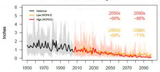
Figure 19. Monthly total runoff projections averaged over the Middle Rogue as simulated by 10 downscaled global climate models and a hydrological model for the historical period (1950-2005) and 2080s (2070-2099) under a low (RCP4.5) and high (RCP8.5) greenhouse gas emissions scenario. Solid line and shading depict the 10-model mean and range, respectively.
