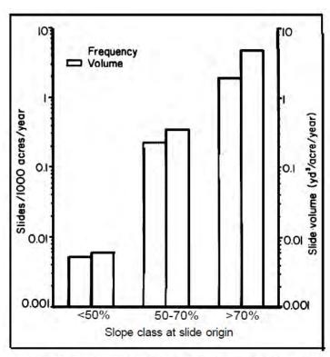
Figure 1. Debris slide frequency and erosion rate on the Siskiyou National Forest, 1956-1976. The rates were strongly associated with slope class.
