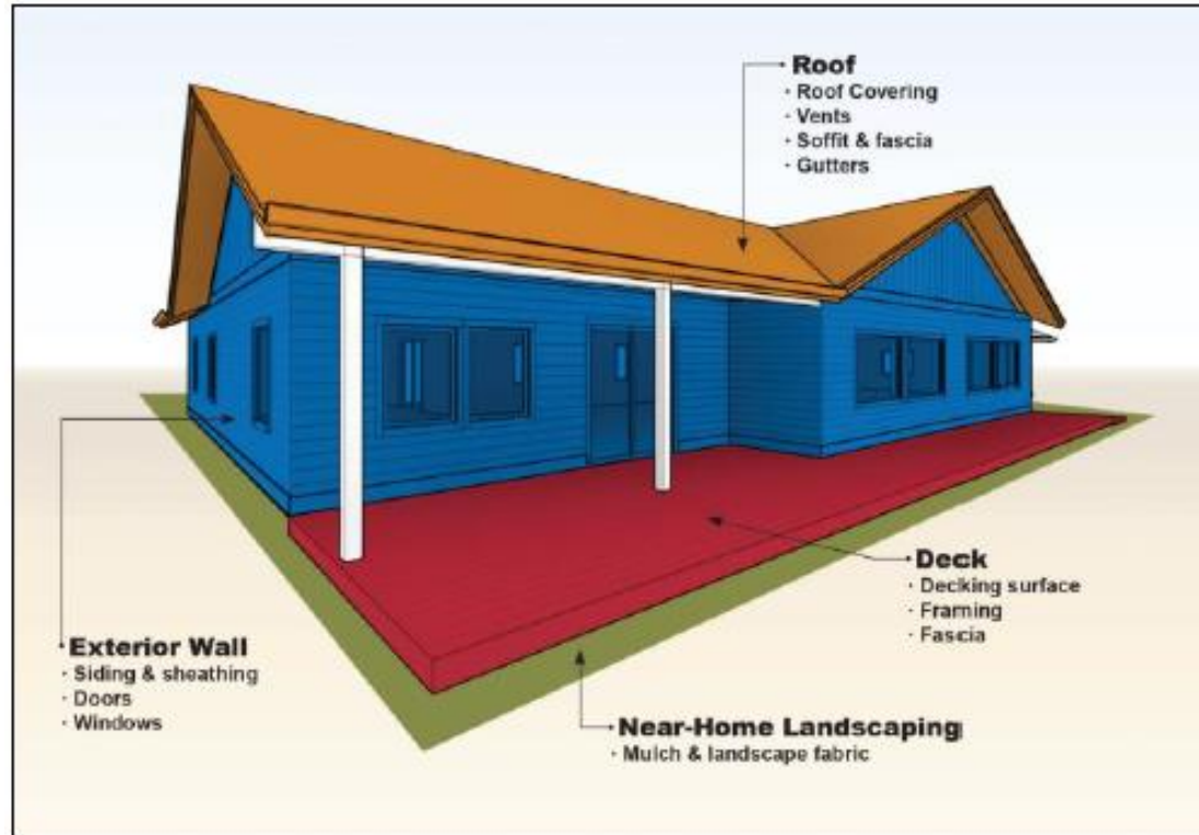
Figure 1. Model home used for cost analysis in this study. It is a three-bedroom, 2,500-square-foot, single-story home representative of wildland-urban interface building styles in southwest Montana.
