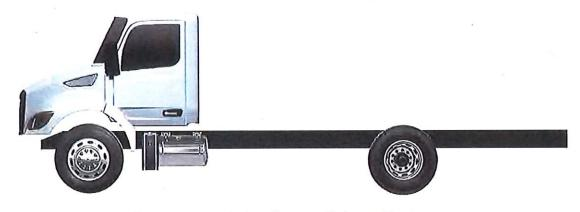
Recommended payload center of gravity to achieve specified ground loads; measured from centerline of drive axles: 54 in. from the centerline of the drive axle(s)."
