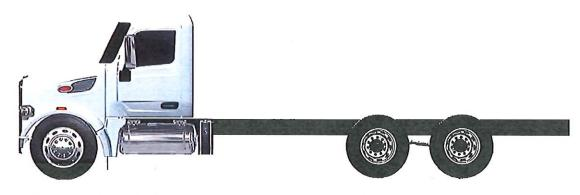
Recommended payload center of gravity to achieve specified ground loads; measured from centerline of drive axles: 51 in. from the centerline of the drive axle(s)."
