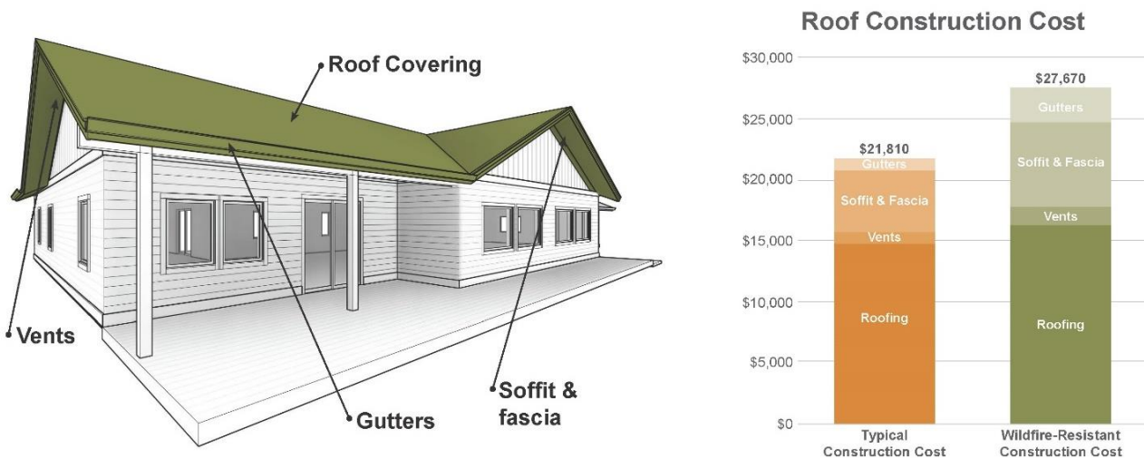
Figure 3. Roof subcomponents and new construction cost.
